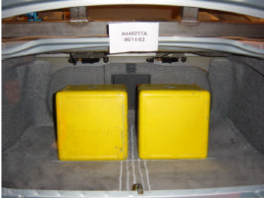
fig. 1: R17 blocks (left) and realistic luggage (right)
