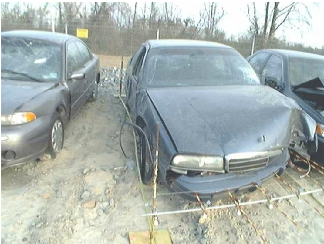
Frontal damage to case vehicle
