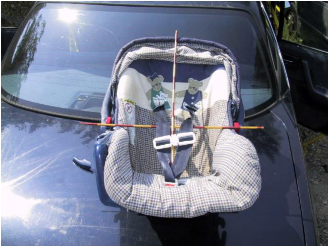
Rearward facing CRS with broken belt guide used by 4 month old child
