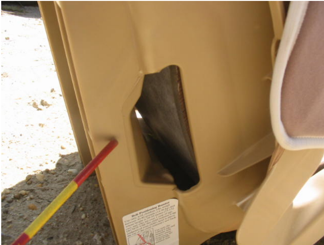
General view showing area of stressing to area around inboard belt guide
