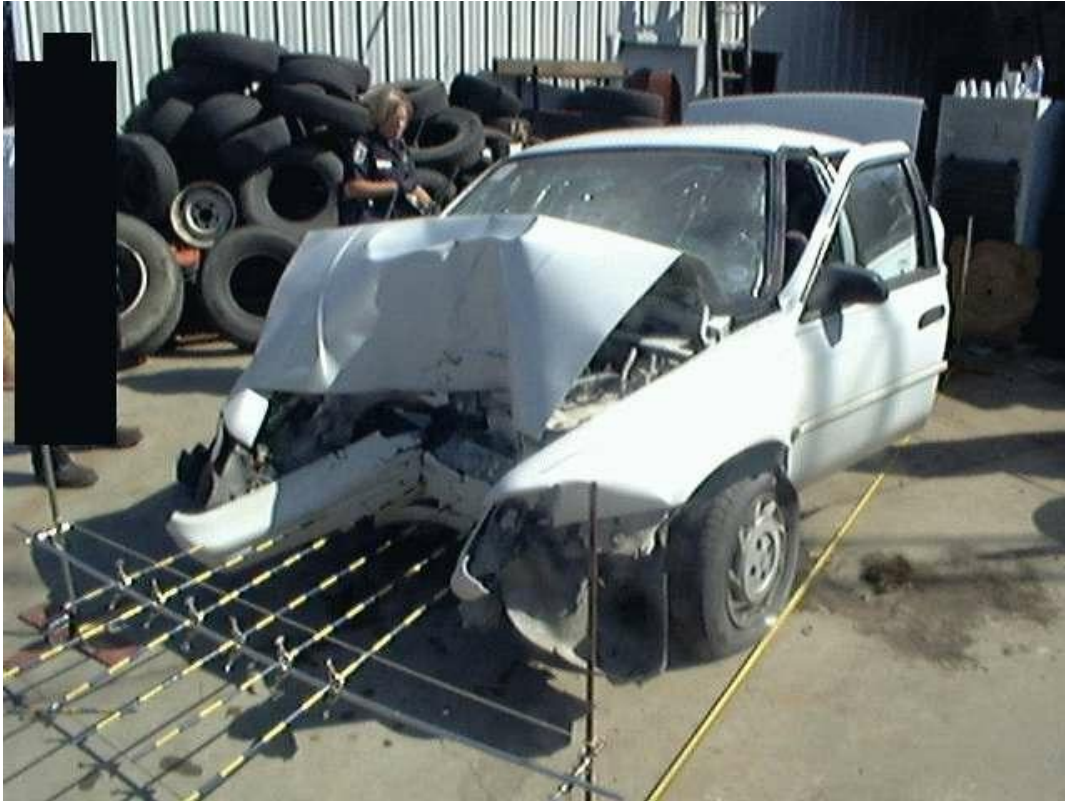
Case vehicle frontal damage
