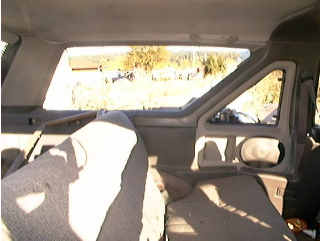
Possible ejection route through rear glazing
