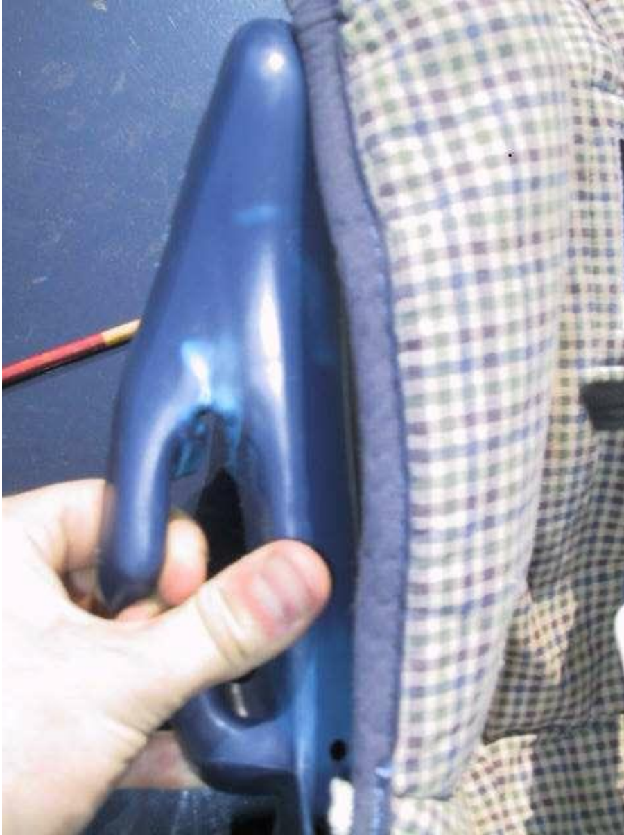
Stressed right hand belt guide
