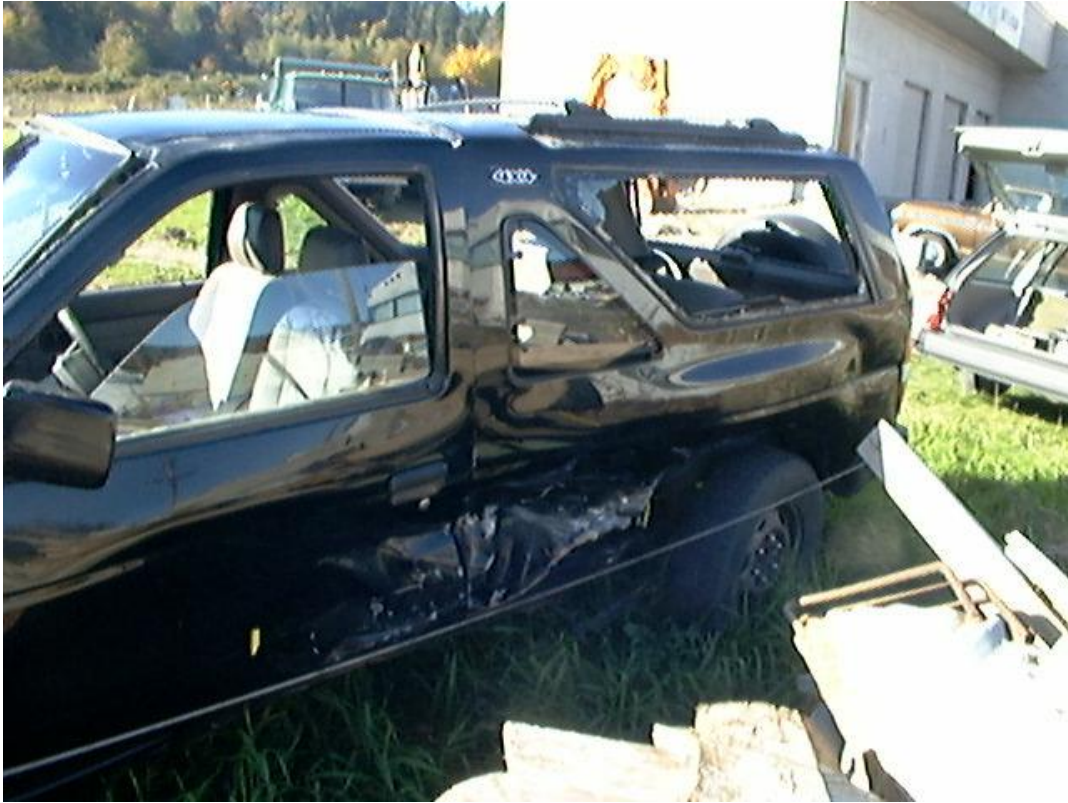
Left side damage to the case vehicle from initial impact with other vehicle
