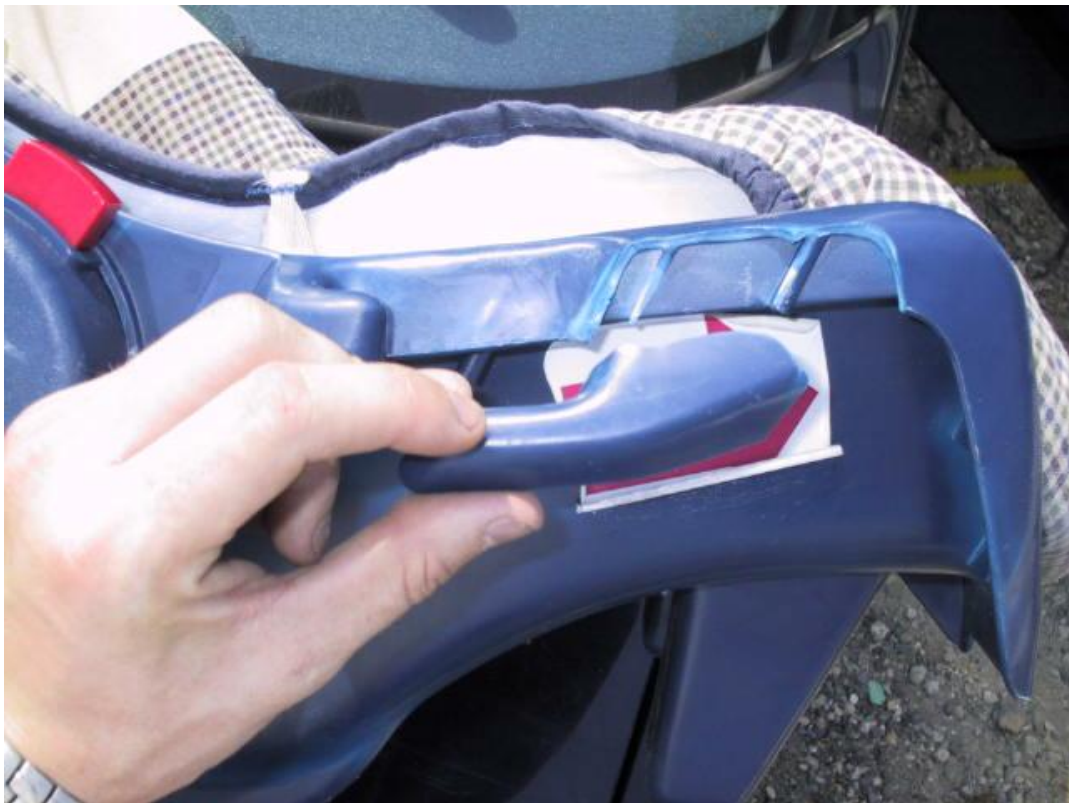
Broken inboard (left hand) belt guide
