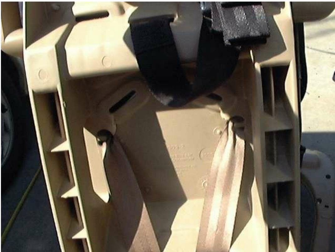
Shoulder harness webbing has cut through seat shell
