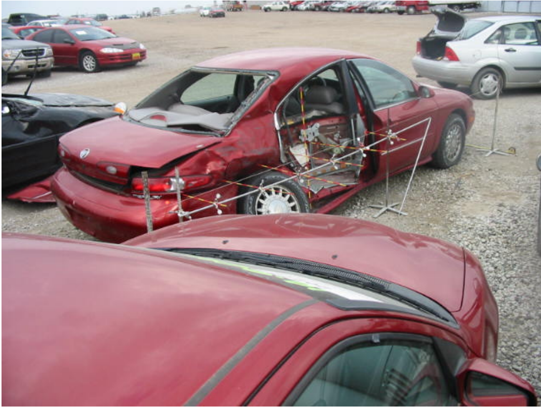
Case vehicle showing damage to right rear
