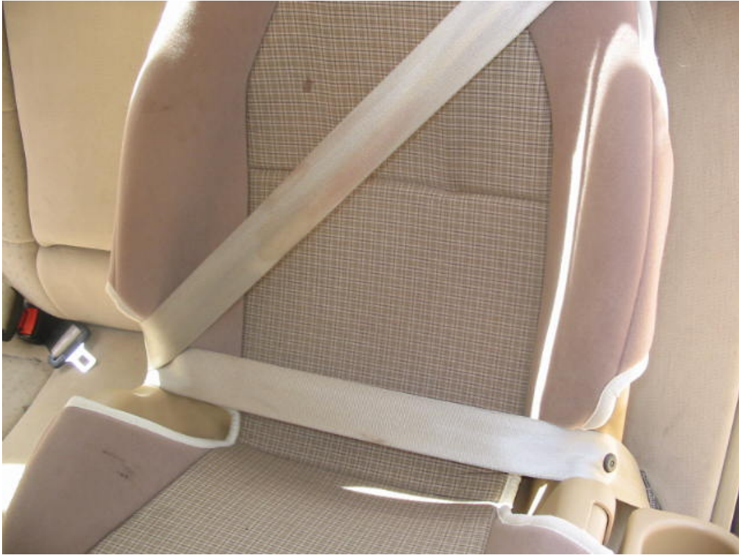
Lap belt geometry – high lap belt
