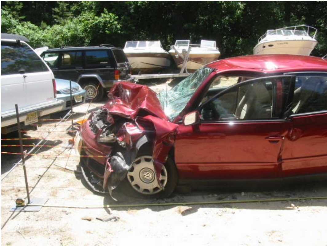
Case vehicle showing frontal damage
