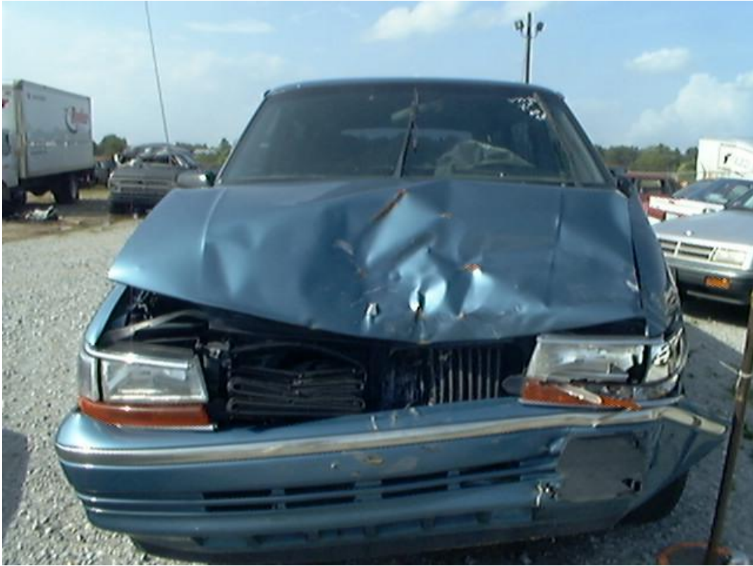
Case vehicle frontal damage
