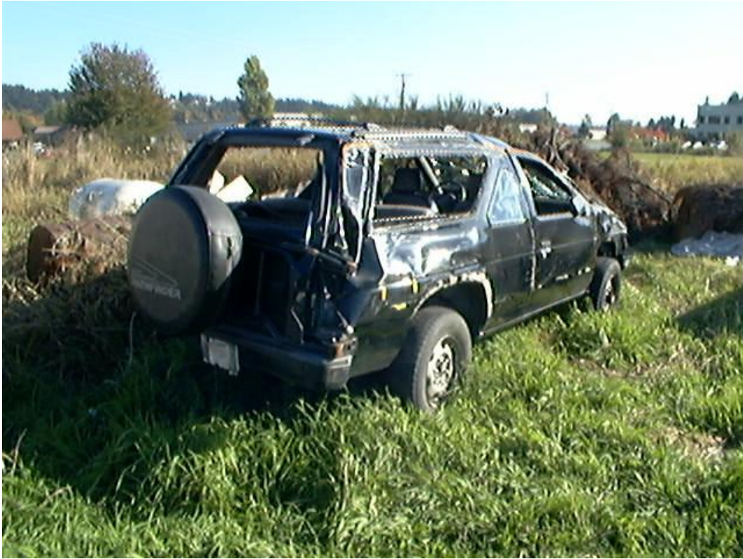
Roll damage to the case vehicle
