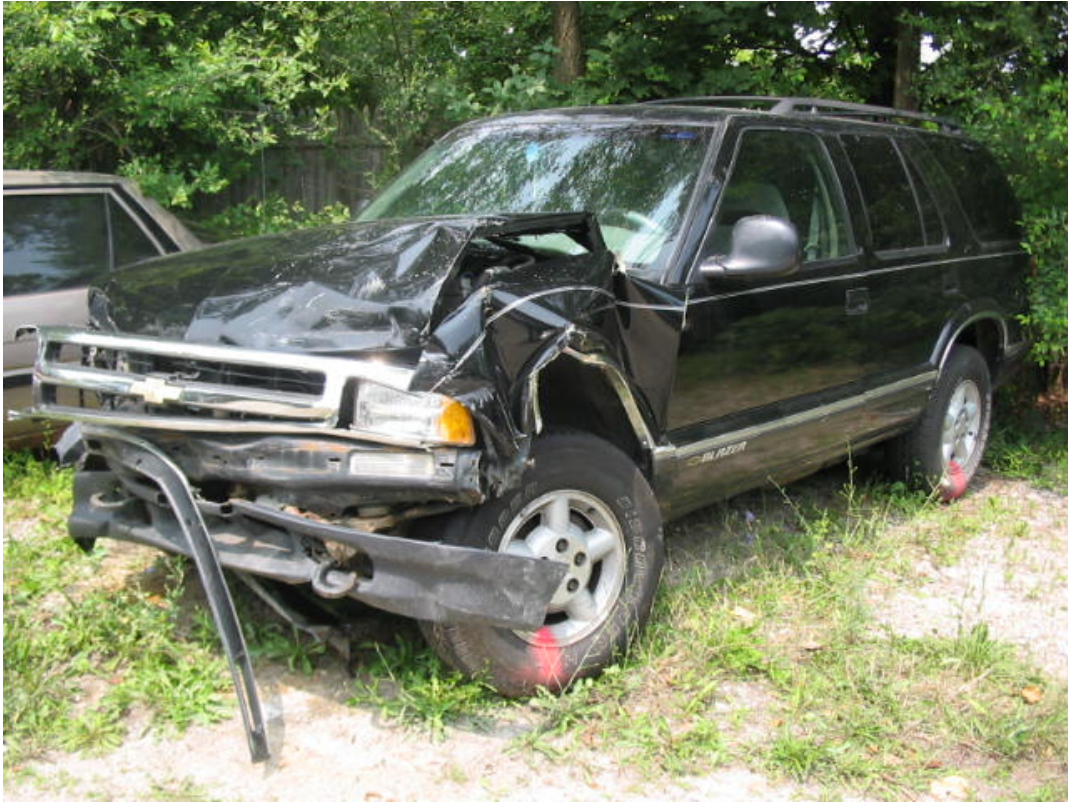
Frontal damage to case vehicle
