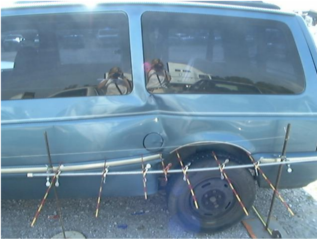
Minor damage to left side of vehicle.
