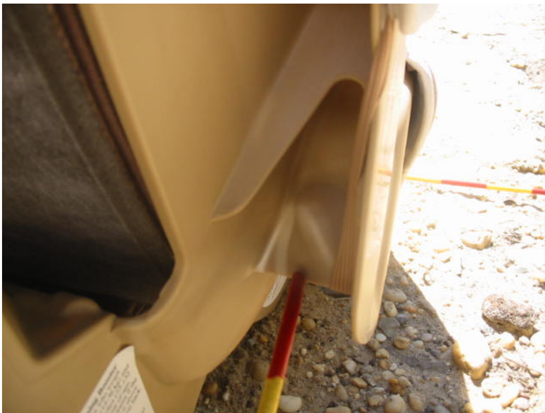
Stressing to area around inboard belt guide
