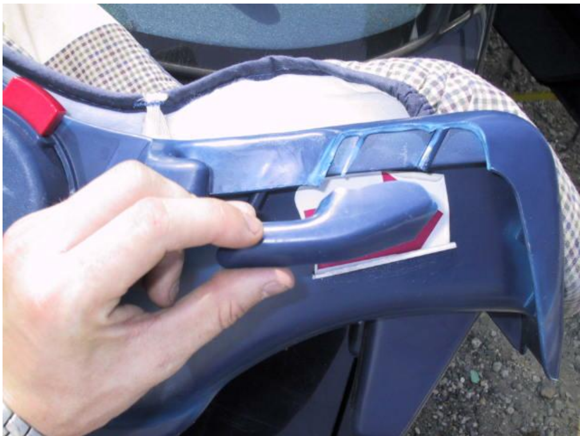
Broken inboard (left hand) belt guide
