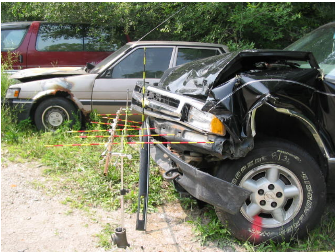
Frontal damage to the case vehicle
