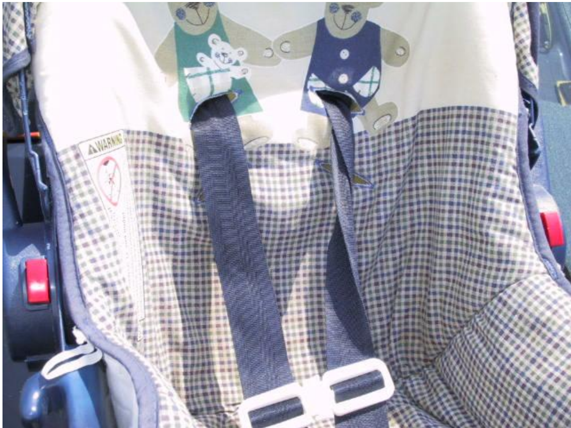
CRS internal harness in highest slots – note: twisted webbing
