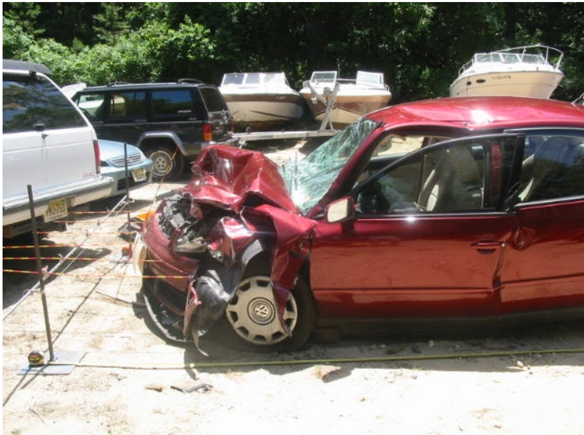
Case vehicle showing frontal damage
