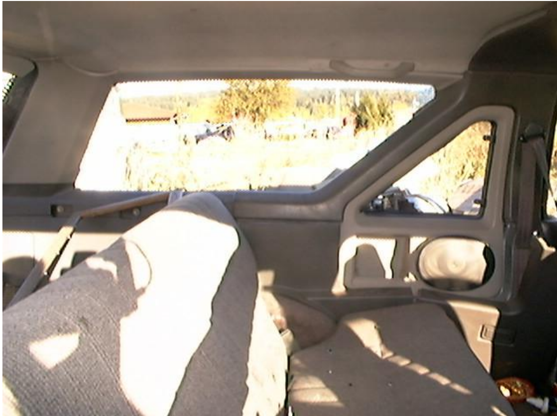
Possible ejection route through rear glazing
