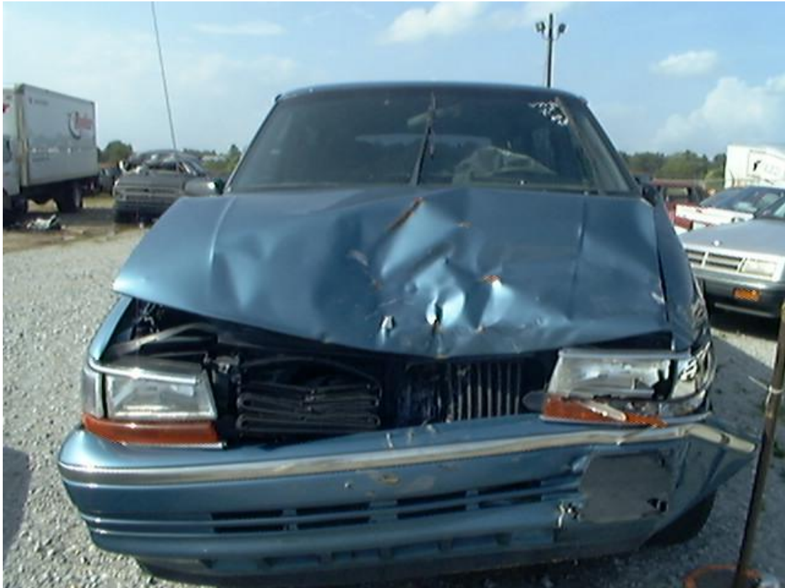
Case vehicle frontal damage
