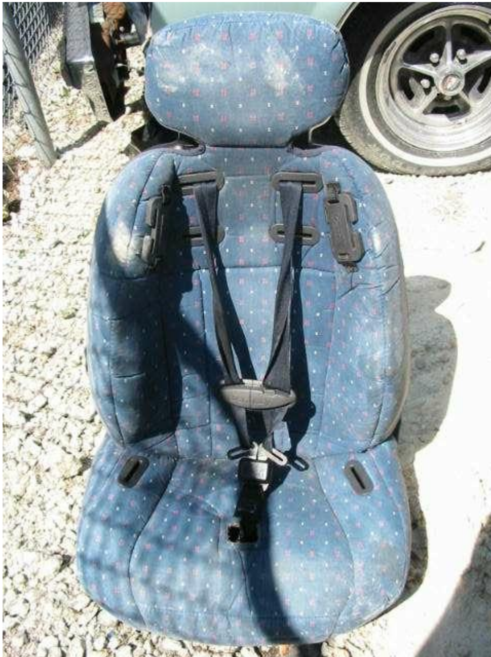
Child seat occupied by two year old child – fractured clavicle. Note the lap sections of the belt do not appear to be properly attached in the photo.
