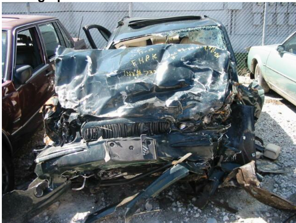
Case vehicle showing frontal damage
