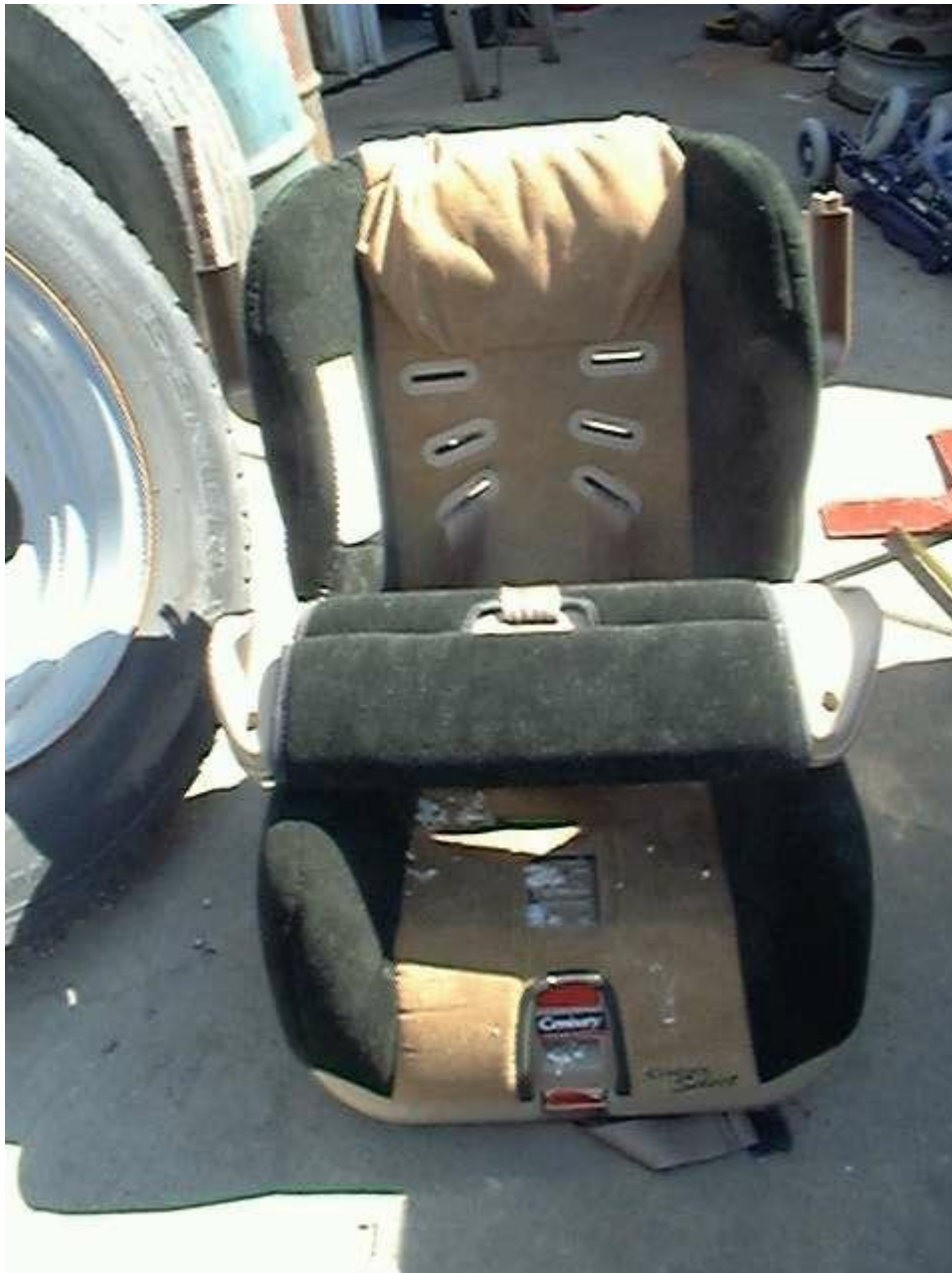
Child seat with broken attachment to shield
