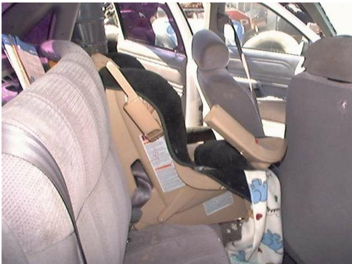
CRS held on lap belt – note broken shield and deformed rear seat back
