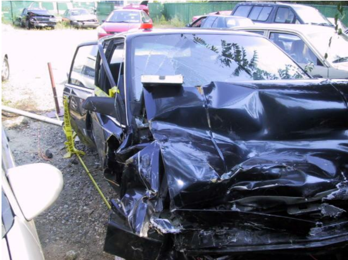
Frontal damage to the case vehicle
