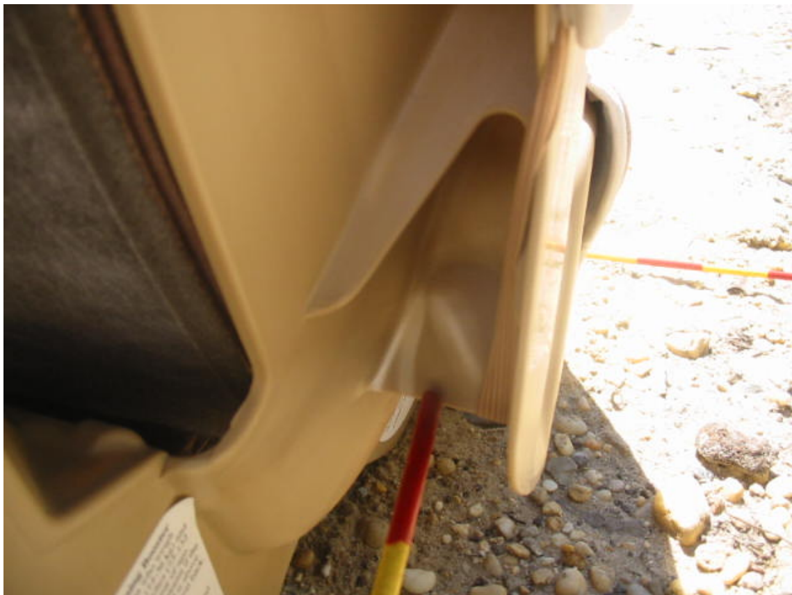
Stressing to area around inboard belt guide
