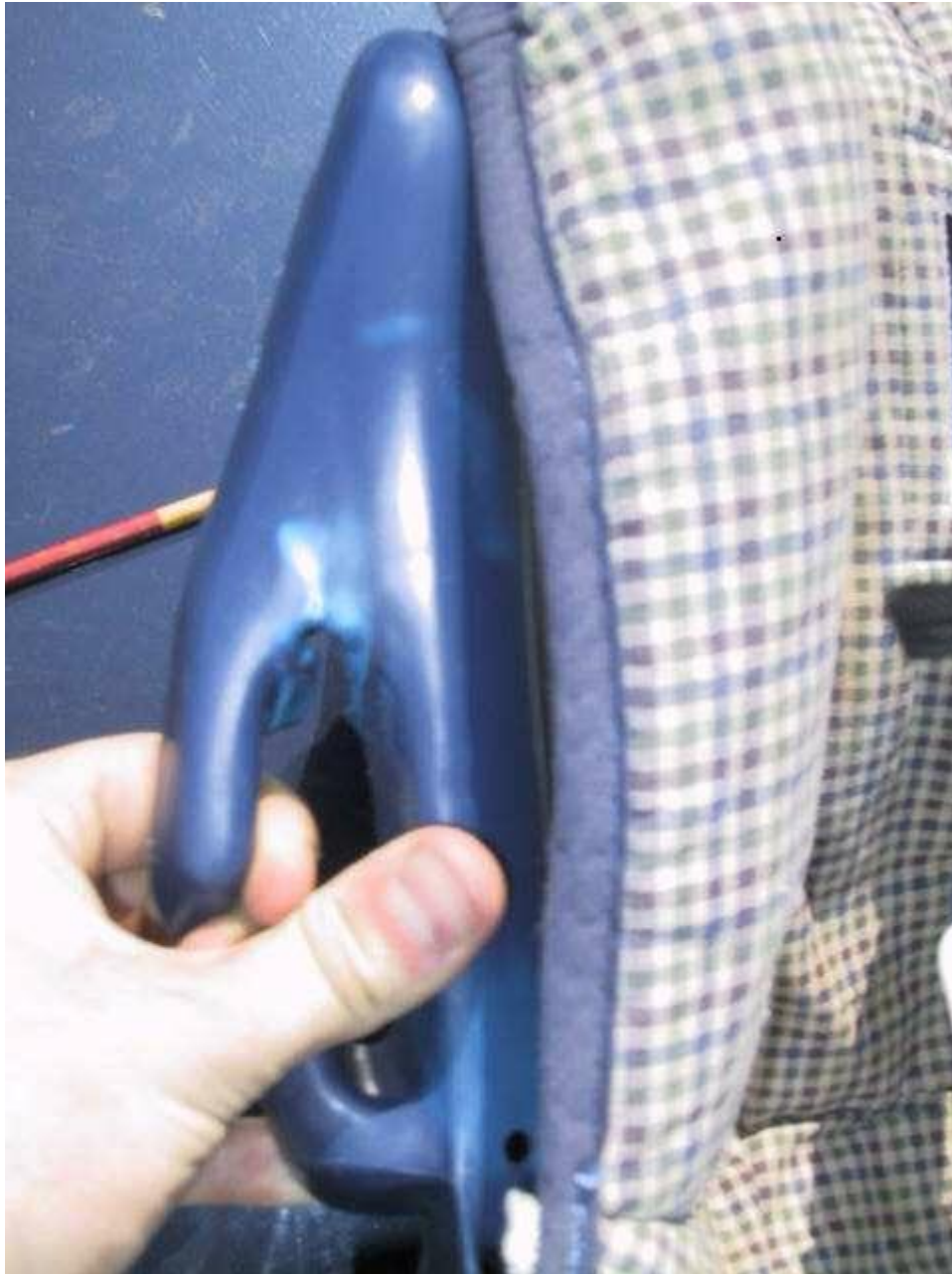
Stressed right hand belt guide
