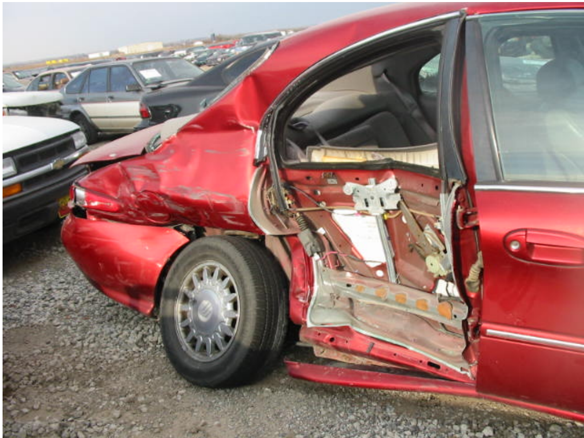
Case vehicle damage to right rear door
