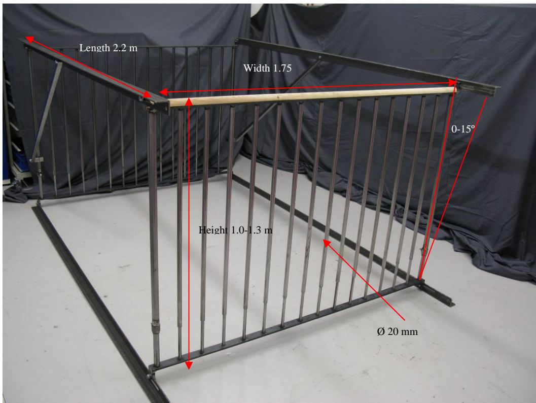
Photo 2.1. The unpainted test rig with vertical bars.
