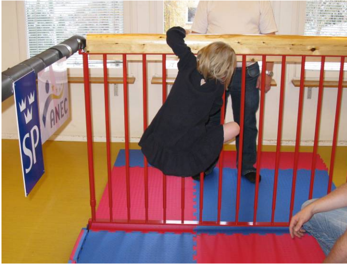
Test barrier C: Vertical bars, height 1.2 m, 100 mm top profile (second attempt)
