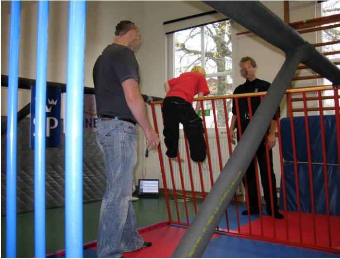
Test barrier E: Vertical bars height 1.2 m, inclined 15° towards the climber (second attempt)
