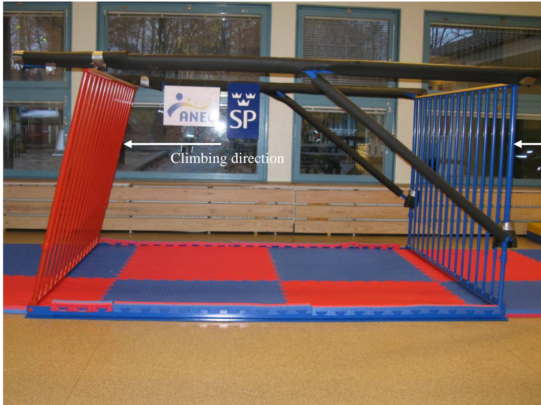
Photo 2.2. The test rig was painted and protruding parts were covered with shock absorbing material.
