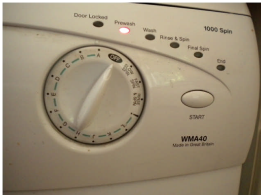
Large bar knob for dialling wash program
