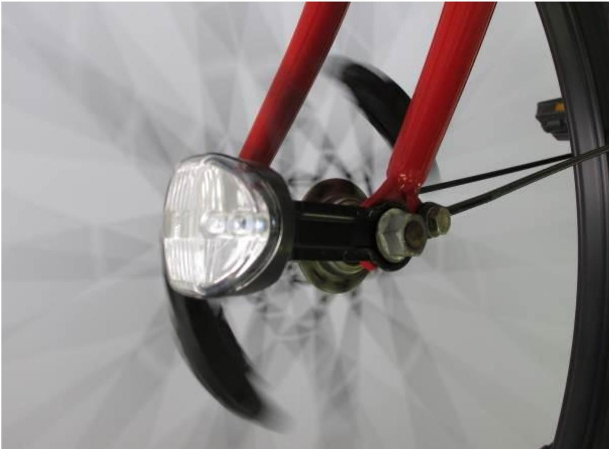
**Figure11: Reelight with a simple dynamo with very low output.**
