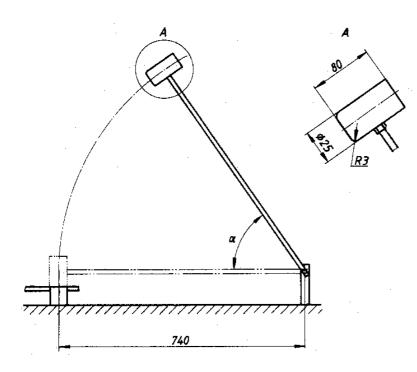
Figure A1 Equipment for impact test.
