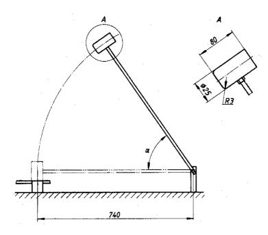
Figure B1 Equipment for impact test
