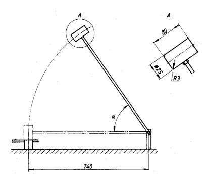
Figure D2 Equipment for impact testing
