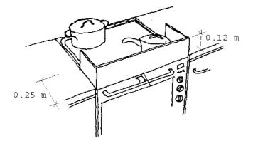
Figure D1 Required dimensions of a hob guard.
