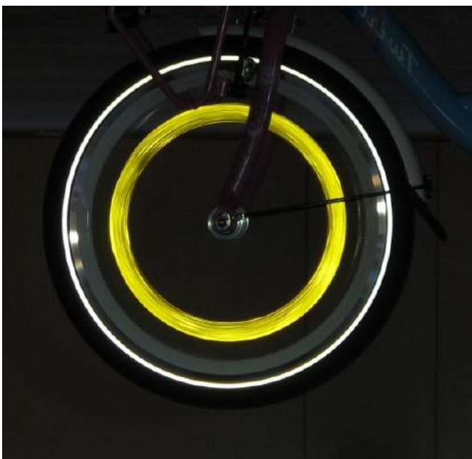
Figure18: The yellow spoke reflection seems to be more visible than the wheel reflector.
