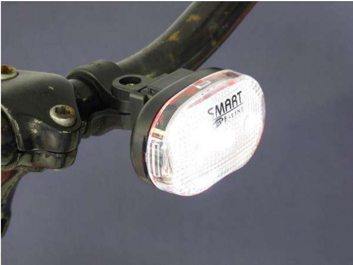
Figure8: Good 'to be seen light' with 2 AAA batteries.
