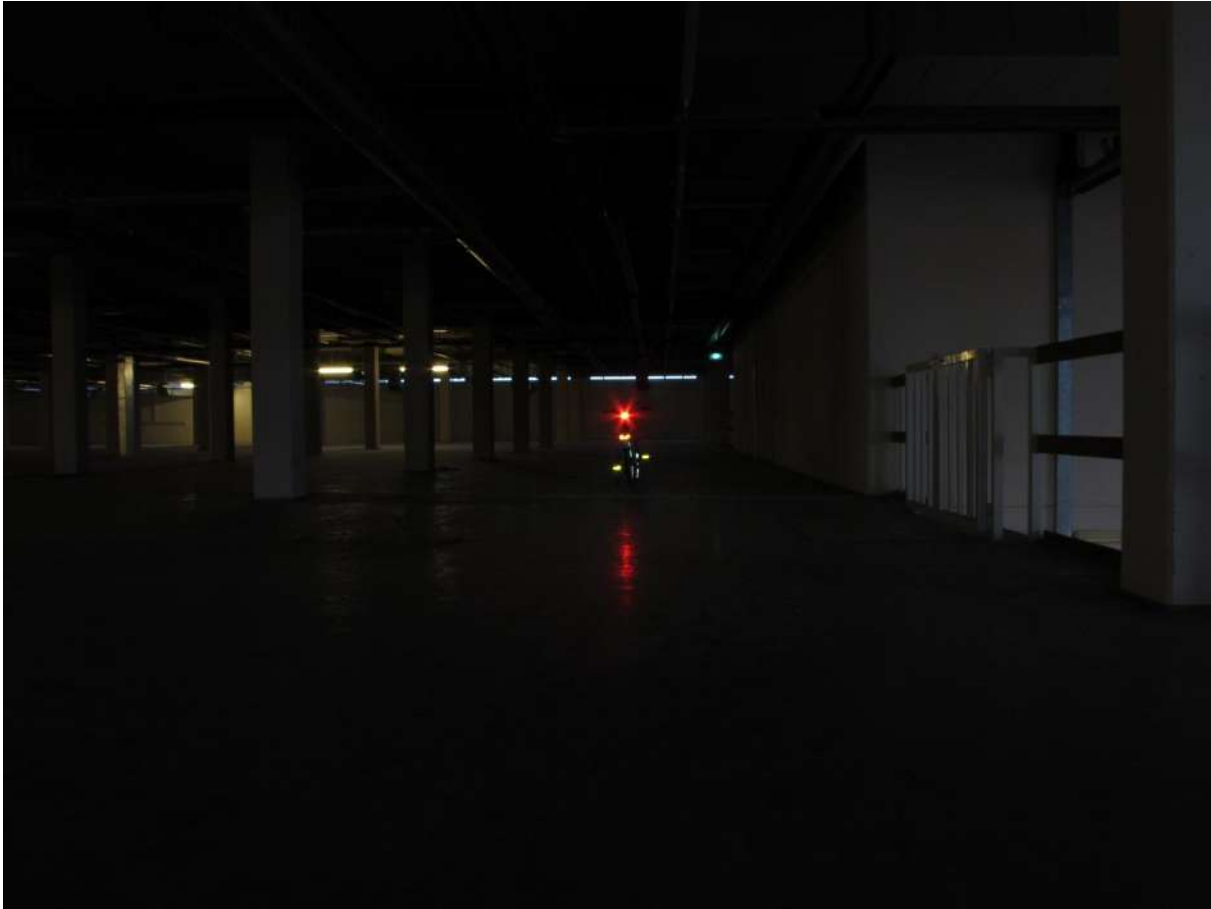
Figure 16: Cheap rear light and reflectors. The reflectors are still visible at close distance.
