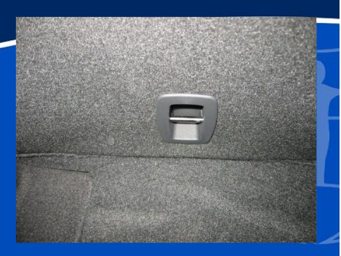
Tether anchorage point appears unmarked
