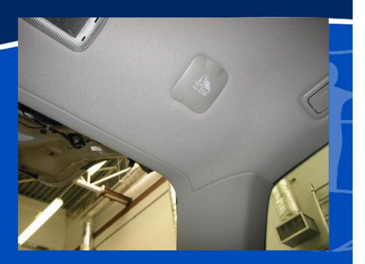
Top tether anchorage, contrasting pictogram on hinged cover in roof line
