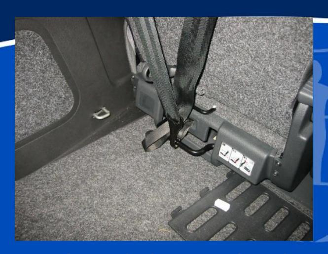
Tether wrongly attached to seat release bar!
