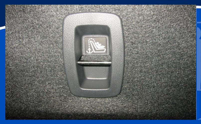
Marking on tether visible from low down
